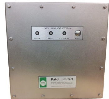
Special Single Zone Linear Heat Detection Cable control panel, with distance location, complete with PSU/charger and battery backup. The panel was for a tunnel application and the specification stipulated it should be able to withstand flooding up to a depth of 3 metres of water. Construction: Stainless Steel 316 - IP68 enclosure.
