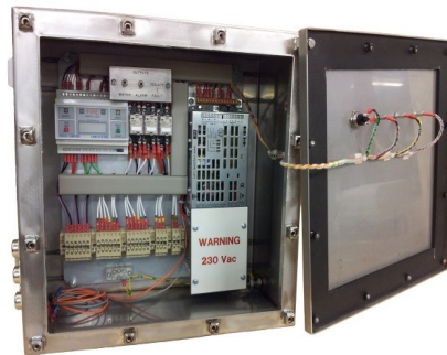
Special Single Zone Linear Heat Detection Cable control panel, with distance location, complete with PSU/charger and battery backup. The panel was for a tunnel application and the specification stipulated it should be able to withstand flooding up to a depth of 3 metres of water. Construction: Stainless Steel 316 - IP68 enclosure.
