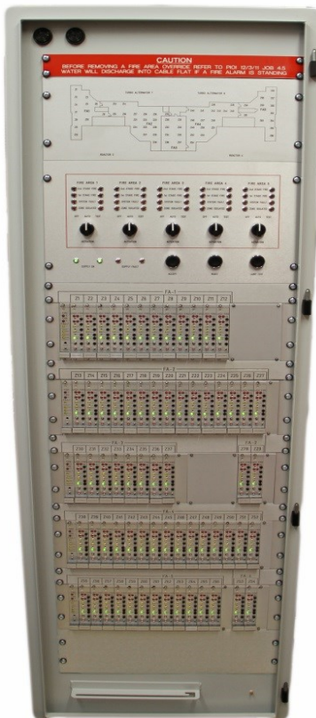
Multi Zone LHDC control panel, complete with sprinkler control Panel and mimic diagram. Construction: Floor standing 19" cabinet with swing frame and glazed door. Application: Nuclear Power Station – Cable Flat Protection
