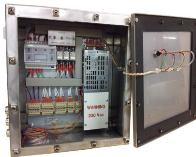
Special Single Zone Linear Heat Detection Cable control panel, with distance location, complete with PSU/charger and battery backup. The panel was for a tunnel application and the specification stipulated it should be able to withstand flooding up to a depth of 3 metres of water. Construction: Stainless Steel 316 - IP68 enclosure.
