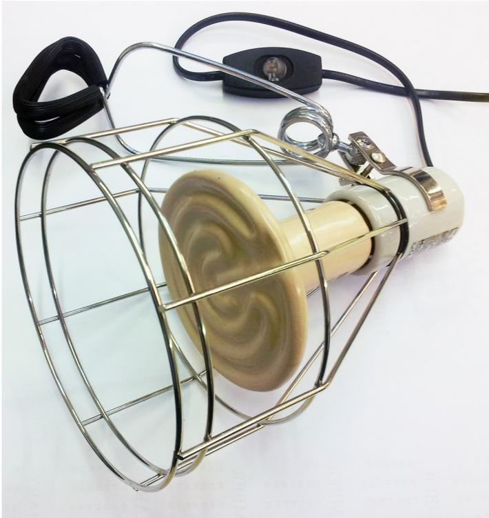
Patols Infrared heat wand is used to test and commission the 5000 series sensors. The wand uses a rapid controllable thermal energy that provides no visible sign of heat, by producing black body Infrared emissions.
