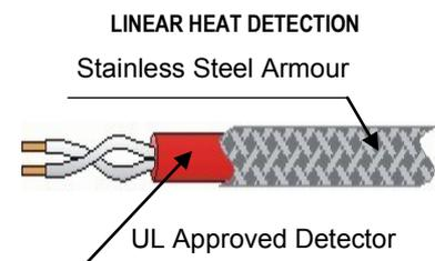
Typical arrangement for *Electrical - Digital LHDC*
