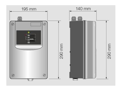
A high-power LED combined with a Large Volume Smoke Chamber (LVSC) results in unparalleled adjustable sensitivity (dynamic range of 0.006%/m to 10%/m) with low aerodynamic resistance and the utmost resistance to dust contamination. These features ensure long system service life and durability.
